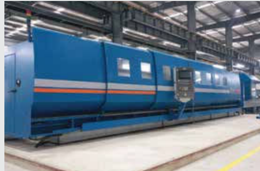
5 AXIS Rotor Cutting Machine Machining Length - Up to 75 mm Dia. - Up to 300 MM
