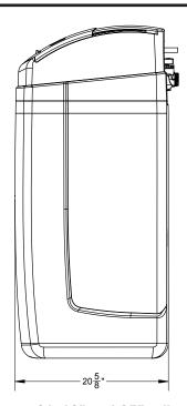
The Water Specialist – CWS-35 Cabinet accepts 35" tall mineral tanks up to a 12" diameter to maximize system capability.
