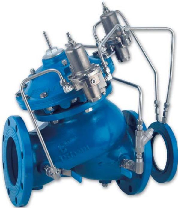
The Model 772-U Flow Control and Pressure Reducing Valve is a hydraulically operated, diaphragm actuated control valve with two independent functions. It maintains both pre-set maximum flow and reduces higher upstream pressure to lower constant downstream pressure, regardless of varying demand or upstream pressure.
